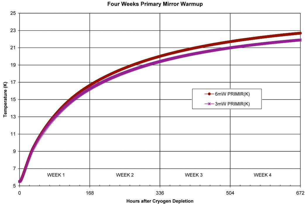
Figure 2. Primary mirror temperature as a function of time after helium exhaustion. (From *CTA Temperature Timelines for Cryogen Depletion*, P. Finley, Ball Aerospace, 23 April 2007).
