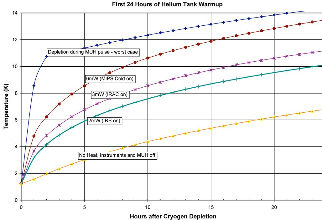
Figure 2. Predicted temperature in the multi-instrument cavity after helium depletion as a function of which instrument or heater is operating. (From *CTA Temperature Timelines for Cryogen Depletion*, P. Finley, Ball Aerospace, 23 April 2007).
