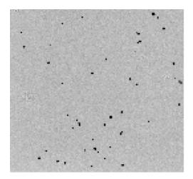
Figure 6.16: Channel 1 IRAC image (100 sec frame time) obtained during IOC/SV. Stars have been subtracted. All the dark pixels are affected by cosmic rays.
