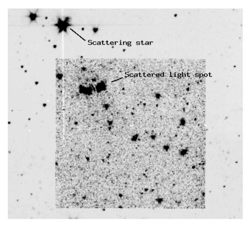
Figure 6.8: Stray light pattern in BCD data when a bright source falls in the stray-light avoidance zone 2A in channel 2. See text and IRAC Instrument Handbook for more detail.
