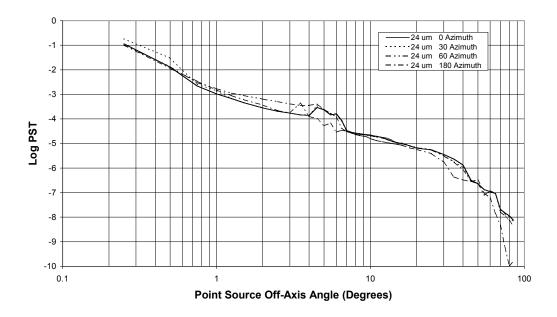
Figure 4.3: Theoretical PST off-axis as a function of azimuth for 24  $\mu m$  .
