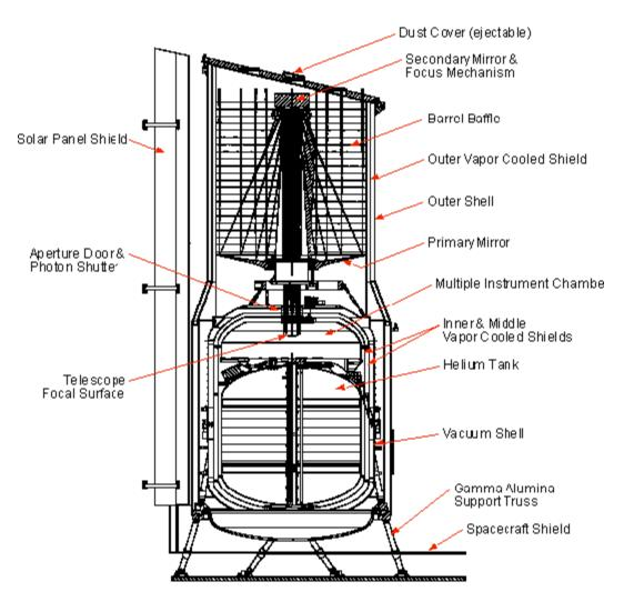
Figure 3.2: Cryogenic Telescope Assembly.
