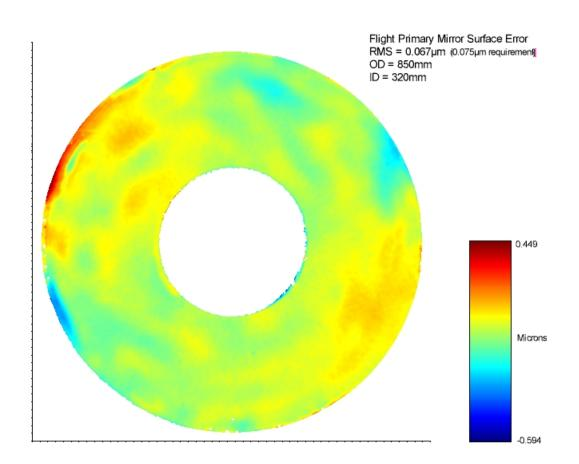
Figure 4.2: The deviations in the flight primary mirror surface. The RMS error was measured at cryogenic temperatures to be 0.067  $\mu$ m rms over the entire clear aperture, meeting the specification of 0.075  $\mu$ m rms.
