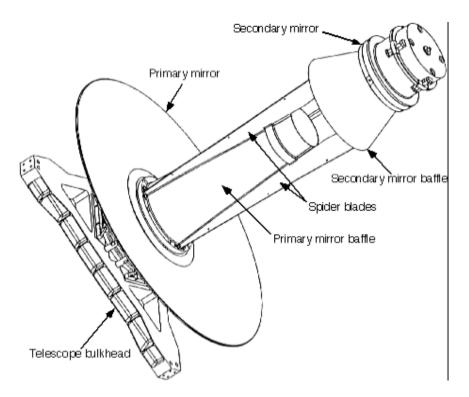
Figure 4.1: Spitzer Telescope Assembly.
