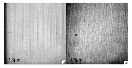
Figure 6.15: IRAC superskyflats for channels 1 and 2 taken during the warm final setpoint calibration. The extended dark spots seen in the channel 2 flat are most likely due to particulate impurities on the pick-off mirror.
