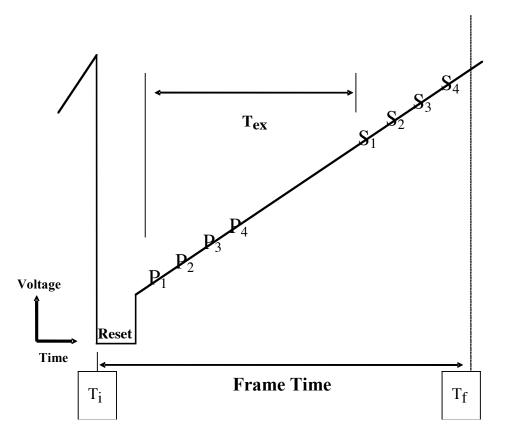
Figure 6.21: Fowler sampling times for one pixel (Fowler N=4). The  $P_a$  (n=1,2,3,4) show the "Pedestal" readouts, and the  $S_a$  show the "Signal" readouts.  $T_a$  is the effective exposure time, and  $T_i - T_i$  is the "frame time," or total time to obtain one IRAC image. The reset part of the sketch is not at the same time and voltage scale as the rest of the figure.
