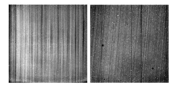
Figure 6.14: IRAC skydark images for the 100 second frametime. The 3.6  $\mu$ m dark is to the left and the 4.5  $\mu$ m dark is to the right. The mean dark levels are 190 and 555 DN. Pixel (1,1), in the lower left corner, is the first pixel read out by the electronics. These images are flipped about the y-axis compared to the BCDs.
