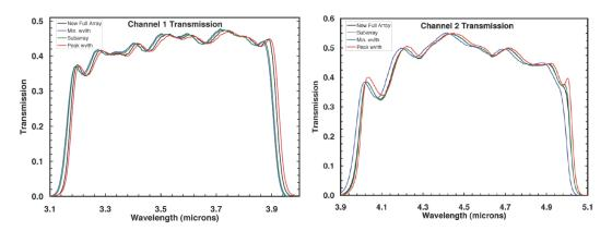
Figure 6.9: IRAC total system response for channel 1 (left) and channel 2 (right), including transmission of the optics and quantum efficiency of the detectors. Digitized versions of these curves are available on the SSC website.
