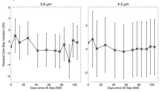
Figure 6.20: Variation with time in the median level of the 12 second warm skydarks at 3.6  $\mu$ m (left) and 4.5  $\mu$ m (right). The uncertainty bars plotted are 1 sigma estimates of the photon noise from the North Ecliptic Pole (lowest background region).
