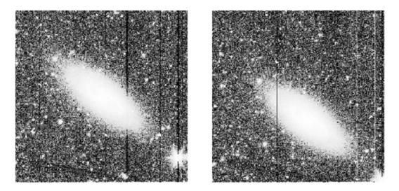
Figure 6.17: Image showing examples of column pulldown and pullup at 4.5 µm. The panels display two sequential 30 second observations of NGC 1353 from the S4G program.
