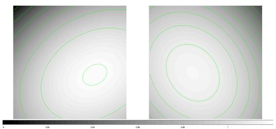
Figure 6.13: Photometric correction images at 3.6  $\mu$ m (left) and 4.5  $\mu$ m (right). The contours start at 0.95 for 3.6  $\mu$ m and 0.94 for 4.5  $\mu$ m and increment by 0.01. The correction images are normalized to the average response of the array.
