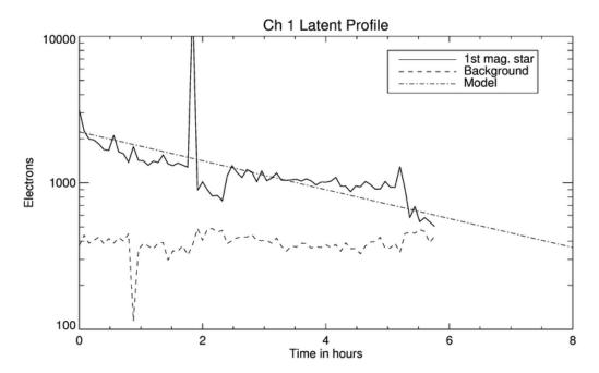
Figure 6.11: Residual image brightness decay as a function of time interval since exposure to a bright source at 3.6  $\mu$ m. The residual is compared to 3 times the noise in the sky background as measured in an equivalent aperture. The fitted exponential decay function is plotted as the dot-dashed line. These curves have been smoothed to mitigate flux jumps due to sources at the position of the original source in subsequent images.
