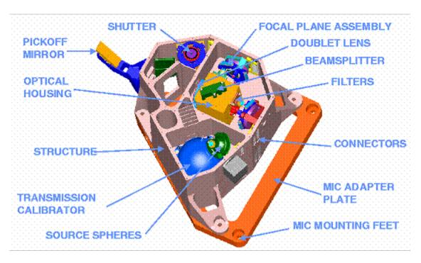
Figure 6.1: IRAC Cryogenic Assembly model, with the top cover removed to show the inner components.
