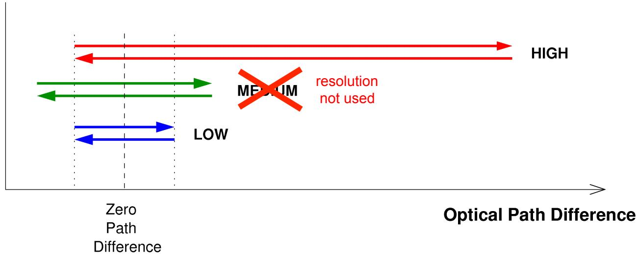
The spectral resolution,  $\Delta\sigma$ , depends on the maximum scan length L:
