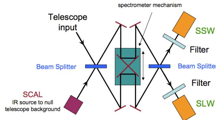
Light from the telescope is split into two optical pathways and interferes with itself at the second beam splitter. Two detector arrays record the light while the spectrometer mechanism moves the rooftop mirrors.
