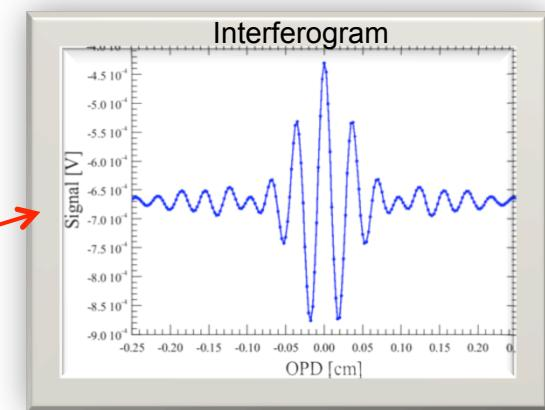
The detectors record intensity versus time. With sensor information from the mechanism this data is turned into interferograms, i.e. intensity depending on optical path difference (OPD). A discrete Fourier Transform turns interferograms into spectra.
