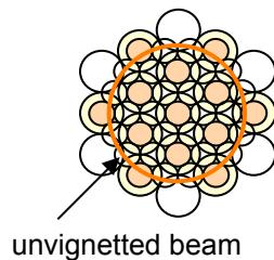
Overlapping spectrometer arrays projected on the sky
