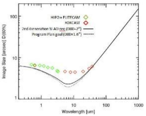
Total image size, including diffraction and anticipated jitter and shear layer seeing, as a function of wavelength.
