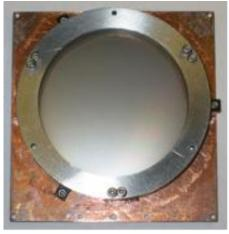
polarimeter (JPL, U. Illinois): in advanced state of development; continuous and stepped rotation of quartz half-wave plates
