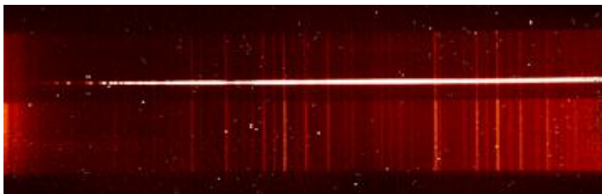
Fig. 8. The spectrum of 69 Leo (A0V) from 1.872-2.346 \mu\text{m} : the spectral trace of the star can be seen in the upper half of the image, corresponding to the narrower (1") slit. Numerous OH lines delineate both slit sections of the mask.
