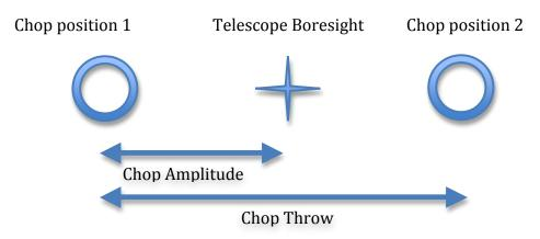
**Asymmetric chopping** means that the secondary is aligned with the telescope boresight in one position, but is tilted away from the boresight in the chop position. The chop amplitude is equal to the chop throw in this case.
