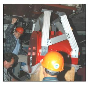
Faint Object InfraRed Camera for the **SOFIA** Telescope (FORCAST) First Science Instrument (SI) to fly this winter
