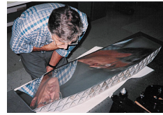
Bernard Bach machined the AIRES grating. Diffraction-limited at 4 μm, it's nearly 4x better than the requirement.
