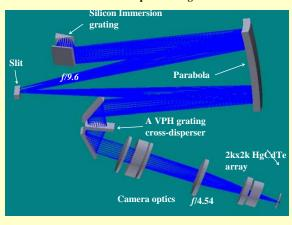
White pupil design Triple-pass parabola as the collimator and lenses camera
