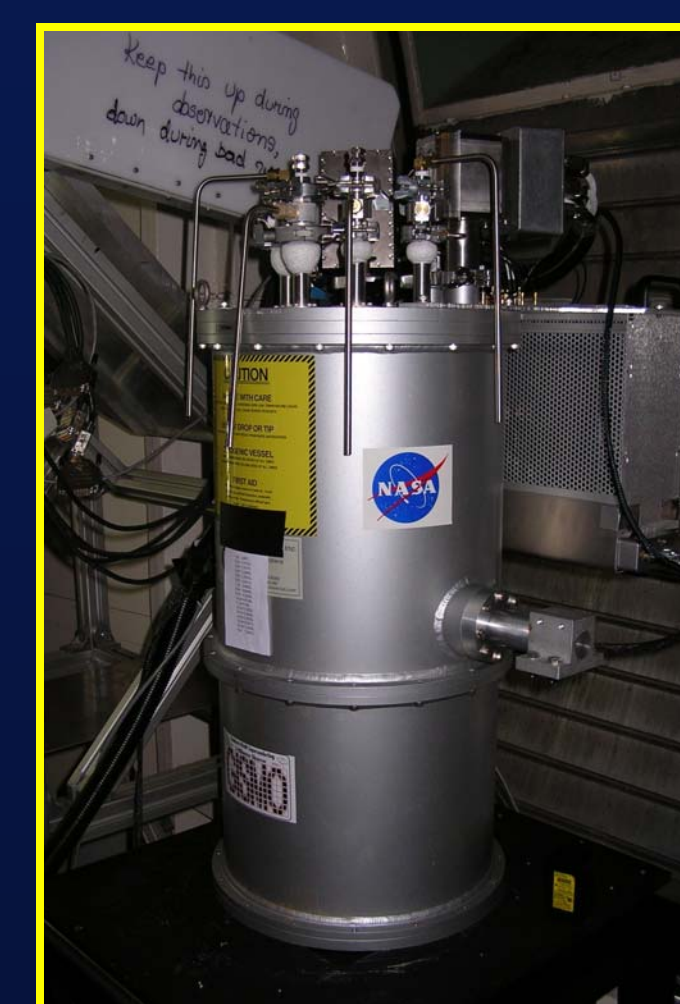
Figure 7. The GISMO dewar at the IRAM 30m telescope.
