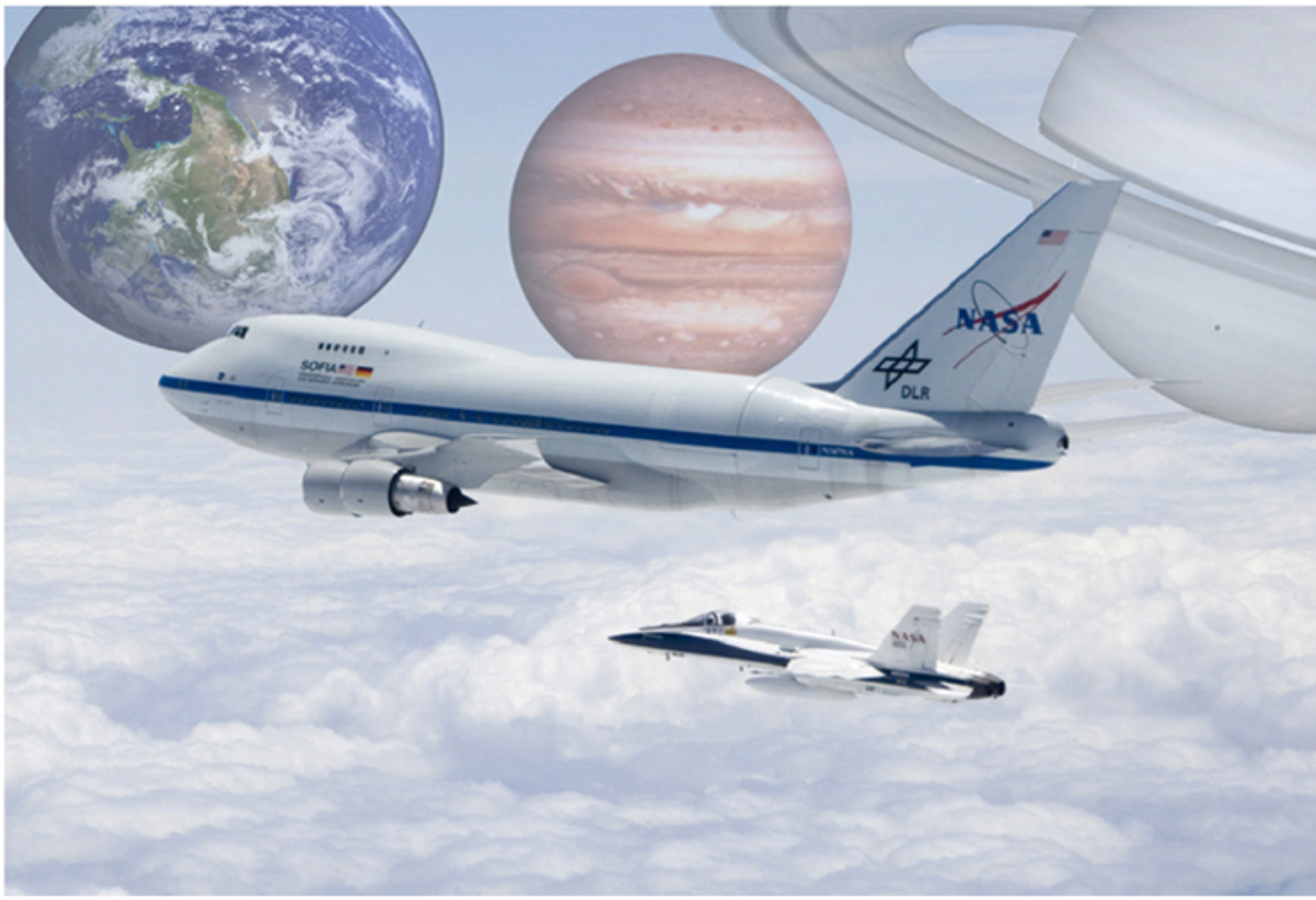
Fig. 1: SOFIA is a NASA partnership with the German Space Agency (DLR) to develop a Boeing 747SP airliner fitted with a 2.7-meter reflecting telescope. SOFIA is the largest airborne observatory in the world, and has had its first light observation in May 2010. On this poster we present the prospects of SOFIA in the field of extrasolar planets.
