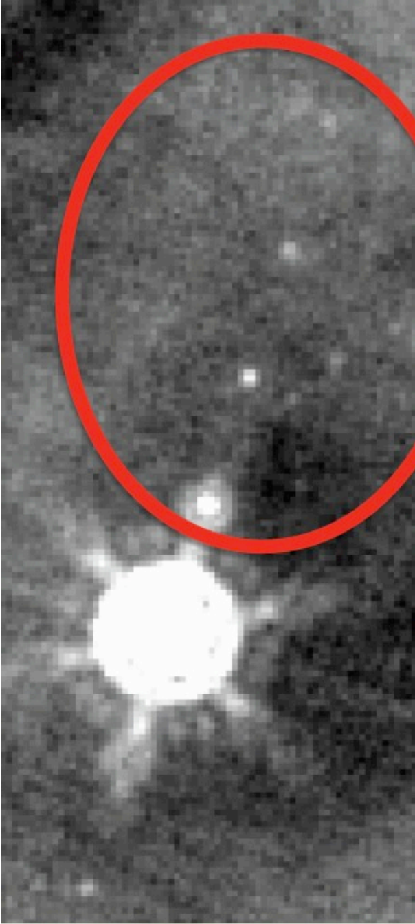
Figure 3.2 Example of MIPS artifacts. Note flatfielding issues and latent images. A new MOPEX corrector module fixes these.
