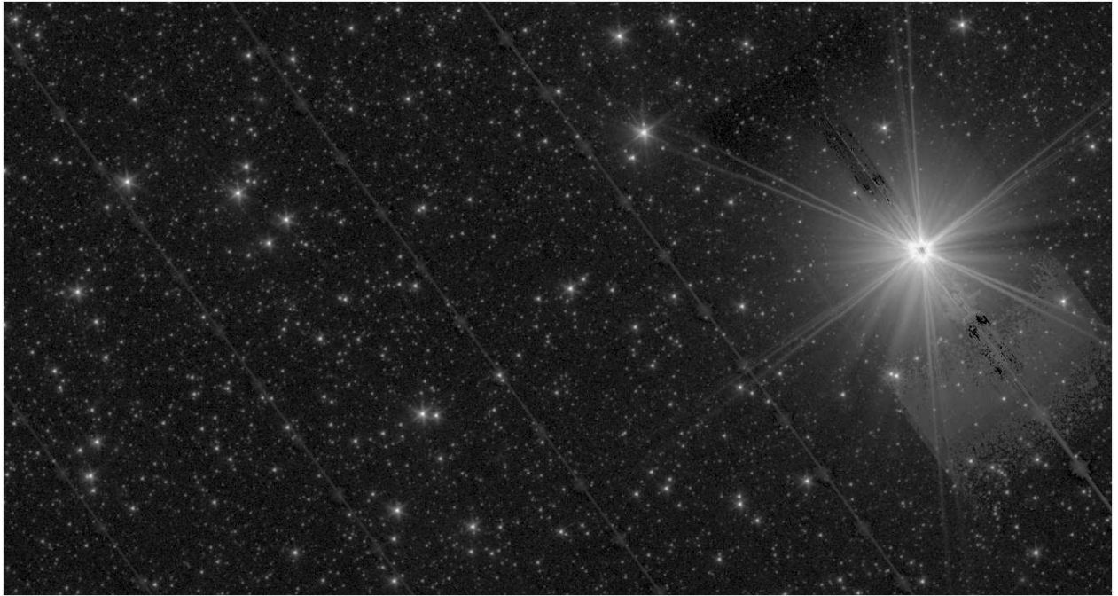
Figure 16: Example of latents (from the bright object on the right) in an IRAC Channel 1 image (centered at l=165.2^\circ , b=-0.45^\circ ). There are also full array pull-ups near the bright source.
