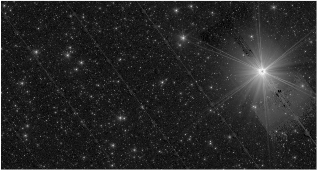
Figure 15: Example of latents (from the bright object on the right) in an IRAC [3.6] image (centered at l=165.2^\circ , b=-0.45^\circ ). There are also full array pull-ups near the bright source.
