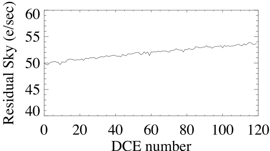
Fig. 1.— The latent charge accumulated in a pixel as a function of time (DCE number). The latent charge was measured in the median of 400 pixels.
