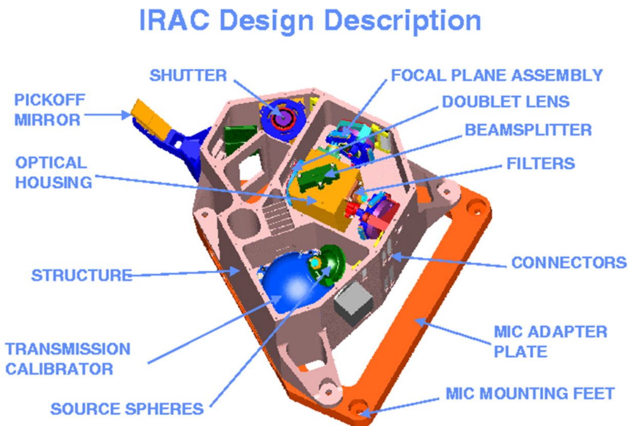
Figure 2.1: IRAC Cryogenic Assembly model, with the top cover removed to show the inner components.
