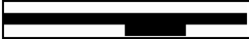
Figure 6.9: Bad pixel mask (pmask) for MIPS-160 data. The centerstripe has no detectors (see SOM for details), and the "bite" in the lower right is the inoperative readout.
