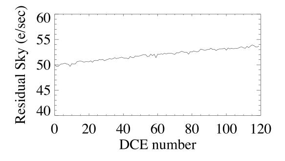
Fig. 1.— The latent charge accumulated in a pixel as a function of time (DCE number). The latent charge was measured in the median of 400 pixels.
